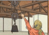
Pulleys can be used to make a small force lift a heavier load. The more wheels in a pulley, the less force is needed to lift a weight.
